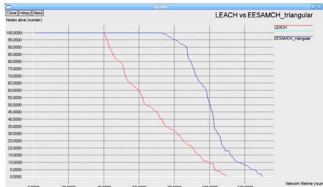
Figure 7: Nodes Alive (Number) vs Network Lifetime (Rounds) for LEACH and the Proposed Algorithm
