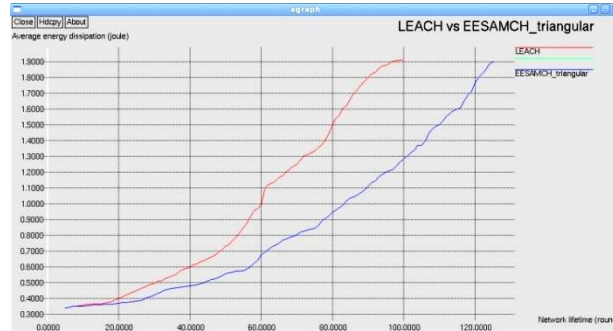
Figure 6: Average Energy Dissipation (Joules) vs Network Lifetime (Rounds) for LEACH and Proposed Algorithm
